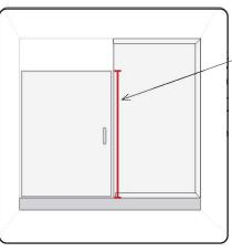
Measure from top of pan curb to top of glass door, trim latch seal and install fixed panel.
